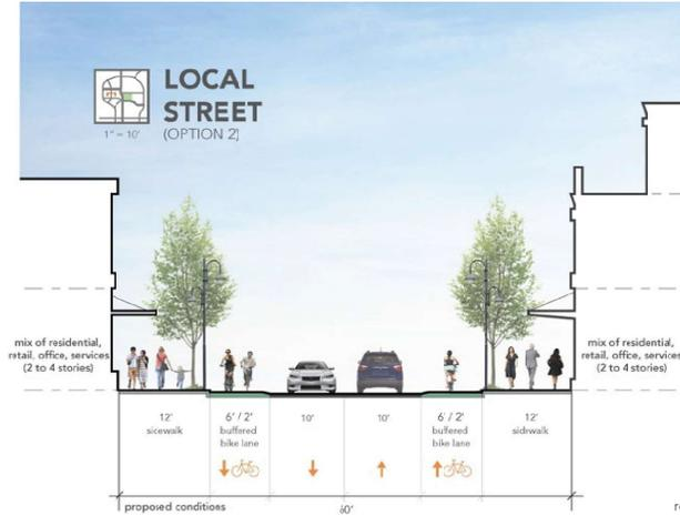
improvements could include reducing the number of lanes through temporary placement of traffic controls using concrete planters or bollards to reduce road width, and restriping for bicycle lanes in the outside travel lane.
