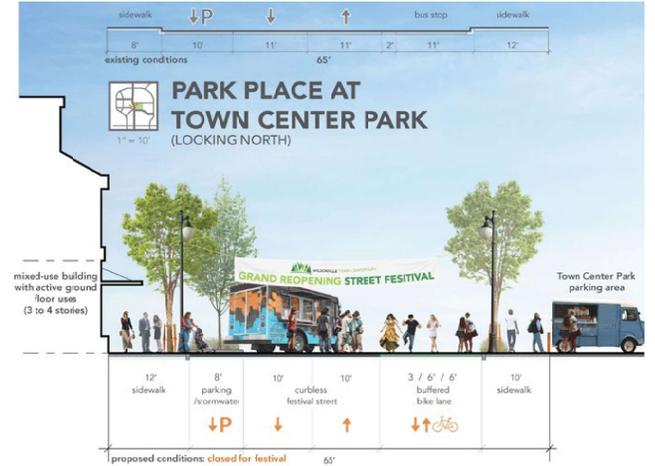
two travel lanes, on street parking, and a protected two-way cycle track, providing an important multimodal connection between the I-5 bike/pedestrian bridge, Promenade, and the two-way cycle track proposed on the north side of Courtside Drive to Memorial Park (see IN.5 for a project description).
