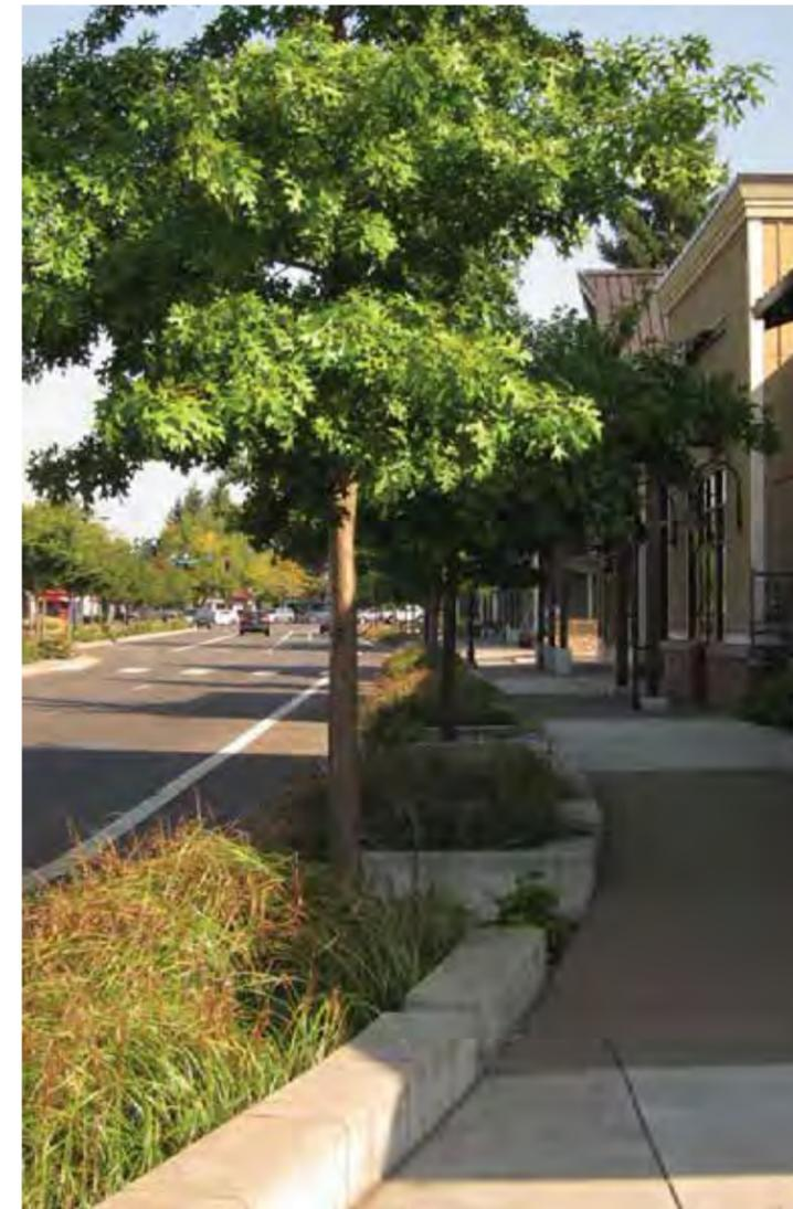
**Stormwater treatment integrated into Main Street**
