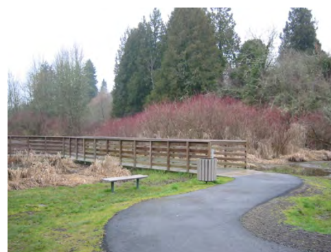
Boardwalks are an appropriate trail design treatment in wetlands or sensitive wildlife habitat areas.
