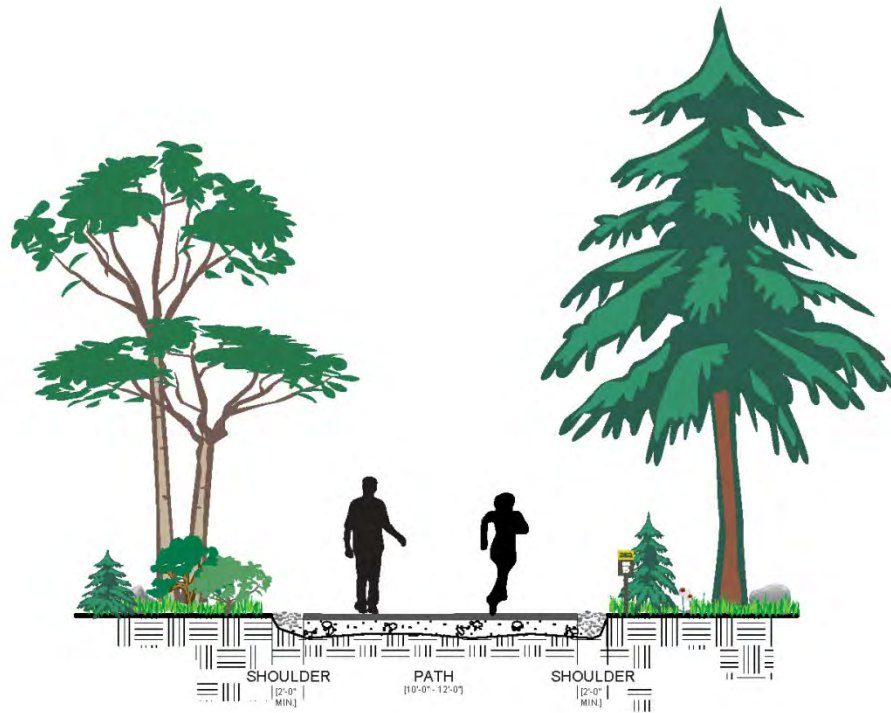
Figure 1 – Typical cross-section for a shared use path
