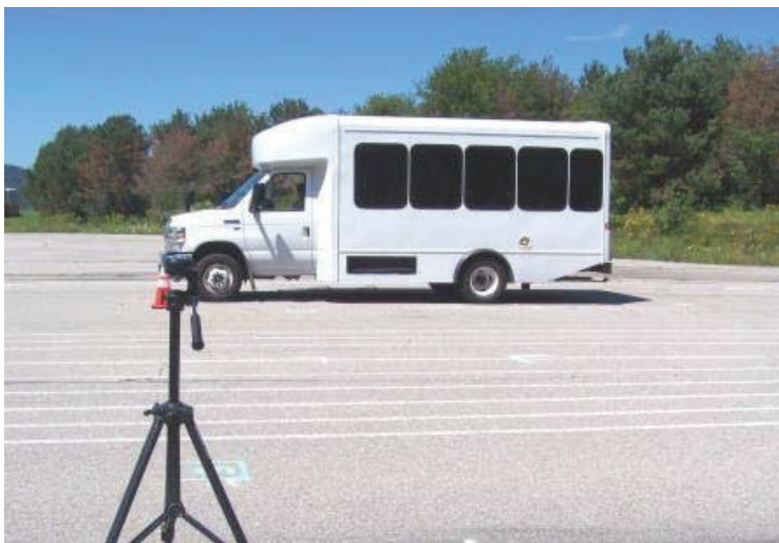
TEST BUS UNDERGOING EXTERIOR NOISE TESTING
