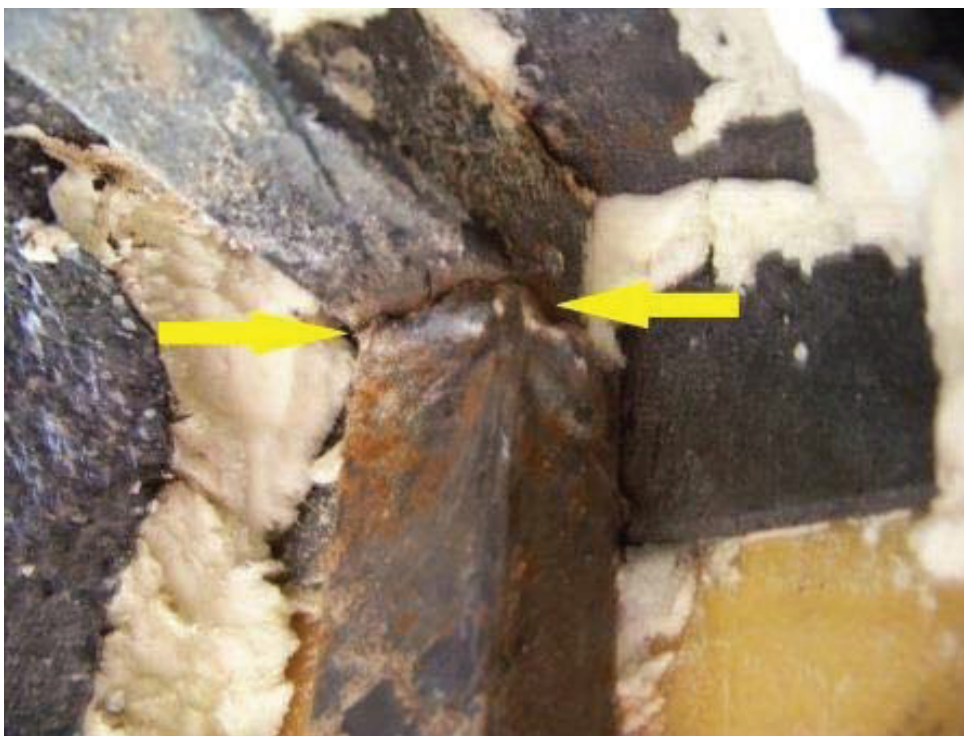
CRACKED LEFT REAR LOWER BODY SUPPORT (1569 TEST MILES)
