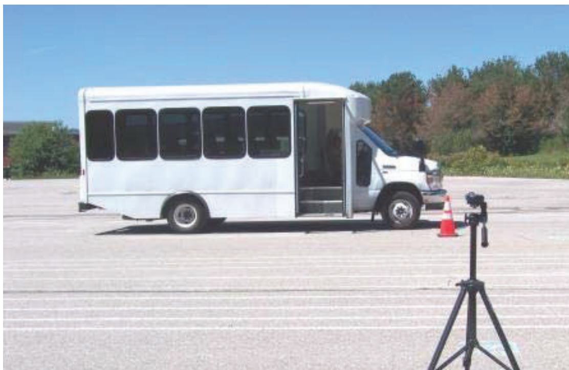
TEST BUS UNDERGOING EXTERIOR NOISE TESTING
