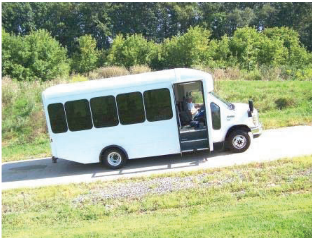
TEST BUS HELD UP AND DOWN ON 20% GRADE
