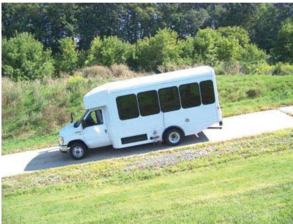
TEST BUS HELD UP AND DOWN ON 20% GRADE
