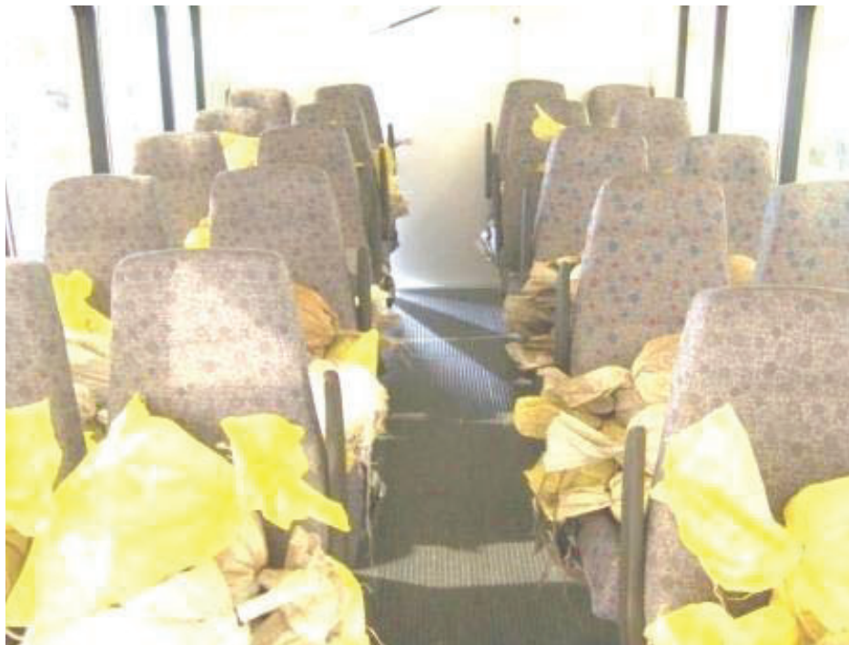
BUS LOADED TO 2.5 TIMES GVL (7,875 LBS)
