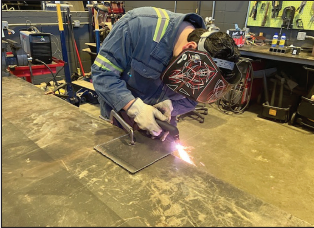
Fleet mechanic Jose Mora fabricating sign brackets for Public Works.
