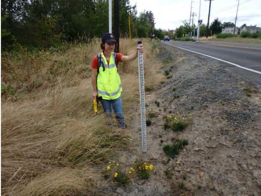
Figure 5. East ditch with sloughing from right bank 2.5 ft height and bottom 2.75 ft width. (node 7)
