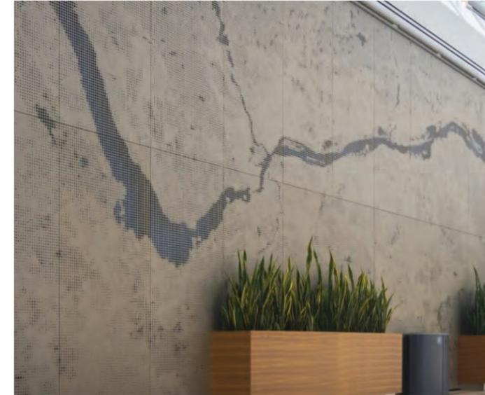
ALTERNATIVE TO ETCHED CONCRETE/CONCRETE FORMLINER WOULD BE A IMAGE/TEXTURE ON PERFORATED METAL.
