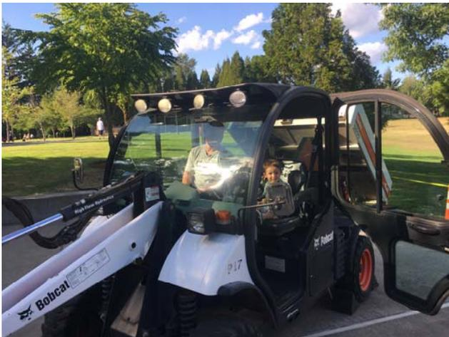
An unusual piece of equipment at the party was the tool cat. This is a multi-use vehicle that can transport work items to hard to access locations, mow difficult terrain with the flail mower attachment and sweep sidewalks/paths with the brush attachment.
