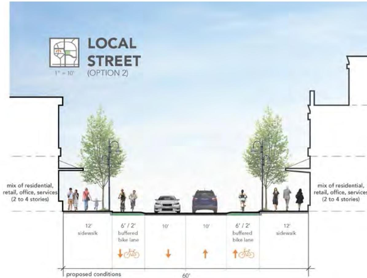
Center Loop W. could also be vacated and right of way used for development. If it remains in place, Town Center Loop W. would be reduced from five to three lanes (two travel lanes with left turn pockets) in conjunction with intersection improvements for Town Center Loop E. to
