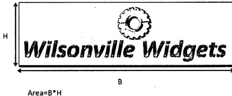
**Figure 1. Measurement of Cabinet or Similar Signs**
