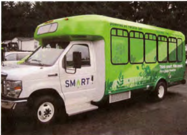
SMART Transit's 21-passenger compressed natural gas (CNG) buses offer a clean burning fuel alternative to traditional diesel buses.
