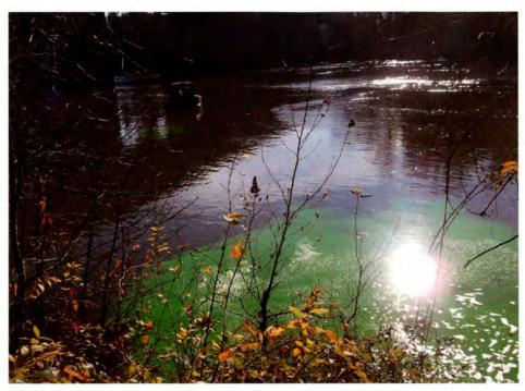
10-November 22, 2013 dye test from the WWTP discharge to Willamette River.
