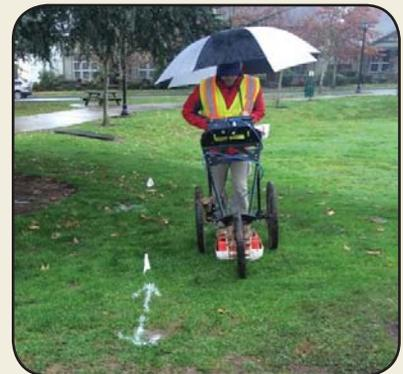
Located irrigation crossover at Palermo Park using Ground Penetrating Radar (GPR)
