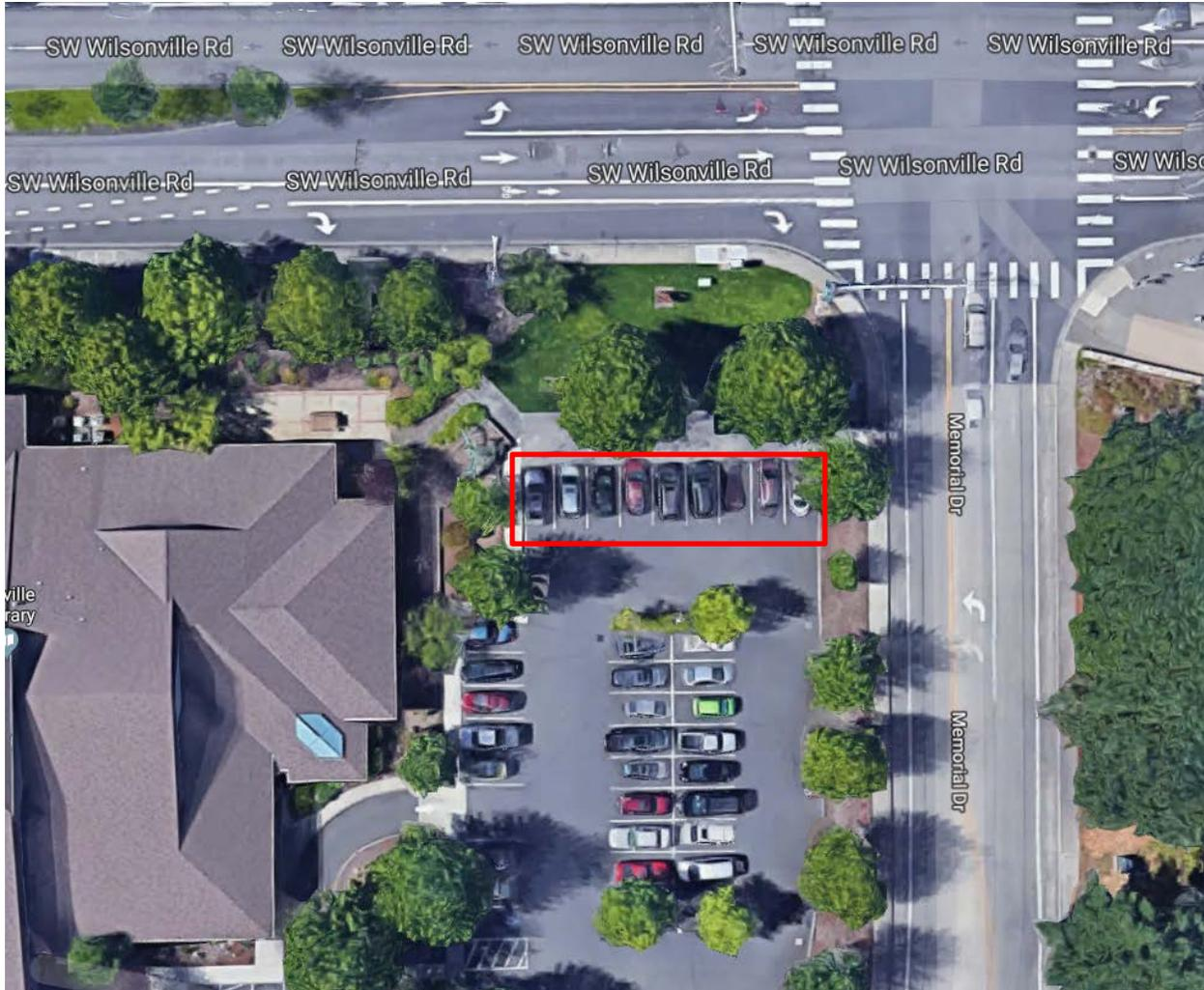
PGE proposes locating the Electric Avenue community charging hub in the northeast corner of the parking lot. The nine existing parking stalls in this area would be converted to six stalls (five conventional, one ADA compliant) capable of charging electric vehicles.
