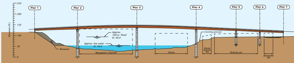
Profile line drawing of Steel Girder bridge
