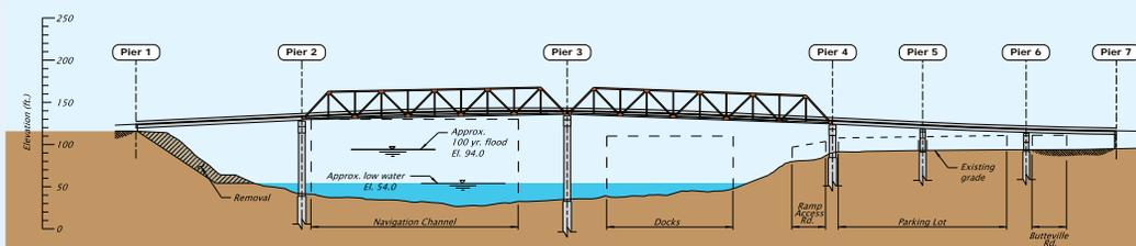
Profile line drawing of Steel Truss bridge
