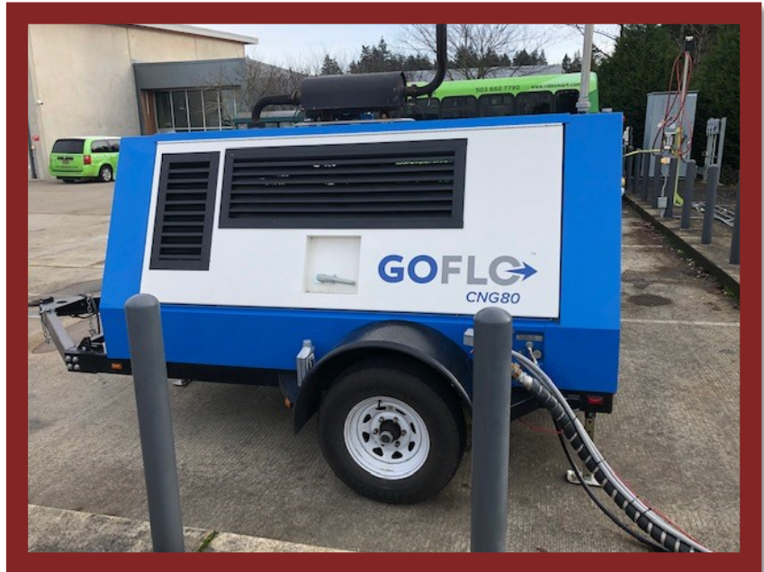
Mobile CNG compressor
