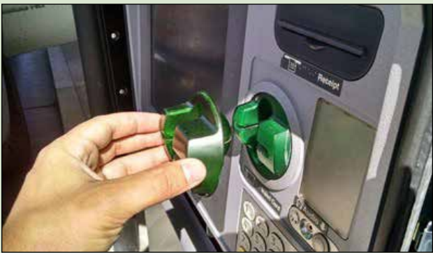
Difficult to detect, digital skimming devices placed at ATMs or point of service can steal credit card data and PIN numbers.
